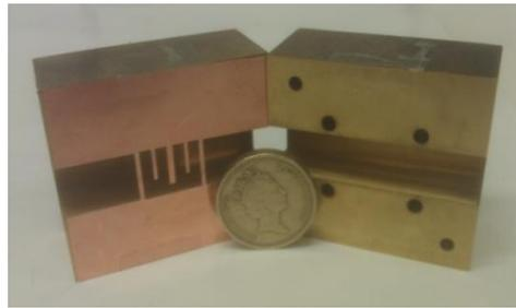
**Figure 3.5-12: Photograph of the fabricated ultra-compact EPS filter insert placed within a channel of a split block waveguide housing.**
