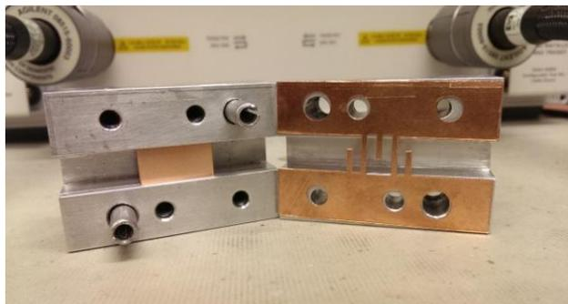
**Figure 4.4-7: Fabricated prototype of the compact 3<sup>rd</sup> order E-plane waveguide filter with source-load coupling.**
