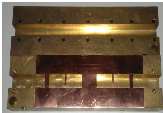
**Figure 3.4-12: Photograph of the fabricated insert for the 4<sup>th</sup> order filter.**
