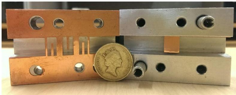
**Figure 4.5-13: Photograph of the fabricated inserts for the compact 3<sup>rd</sup> order cross-coupled filter, placed within the custom made split block waveguide housing.**
