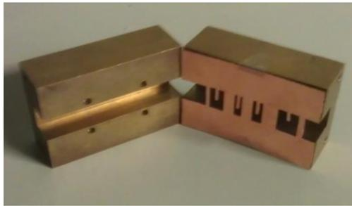
**Figure 3.3-8: Photograph of the fabricated insert for the 4<sup>th</sup> order EPS filter, placed within a channel of a split block waveguide housing.**
