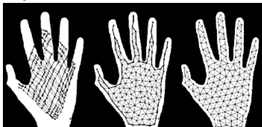
Figure 5. Adaptation process with Kohonen maps, NG and GNG obtaining the contour neurons from the 2D input space of the hand
