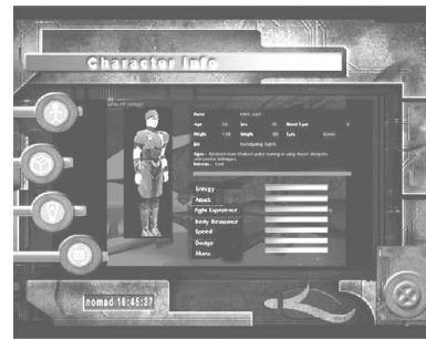
Fig 5: Example of interface redesigned to be more compatible with expectations, created by Vi Bang, Westminster Student. The buttons were designed to be intuitively connected with their function and remained in the same place on consecutive screens.
