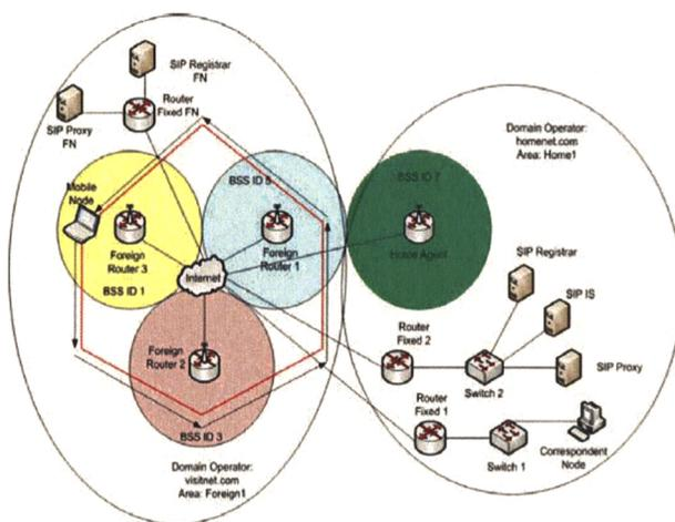
Figure 2. Scenario for Mobile IPv6 - SIP simulation
