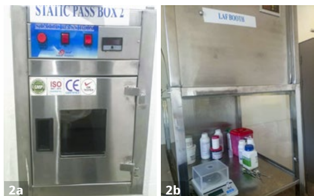
Figure 2 Ruharo Mission Hospital eye drop production facility a. Static pass-box for UV sterilisation of items. b. Laminar air flow booth to weigh ingredients and materials under aseptic conditions.
