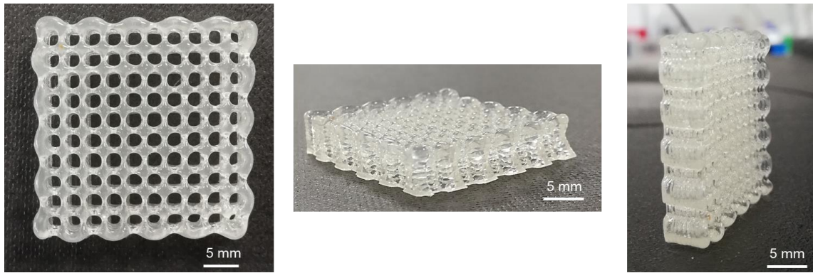
Figure 6.5 3D printed scaffolds of P(3HO-co-3HD-co-3HDD) with 6 mm of height obtained by deposition of 22 layers of material.
