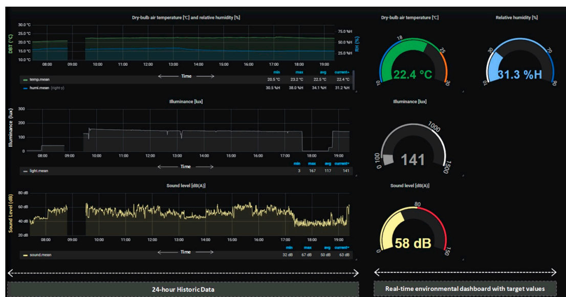
Figure 11. DBT, relative humidity (RH), Illuminance and Sound levels—Real-time IoT data visualisation in the Print Office (source: IoT data display in Grafana tool, edited by the author).
