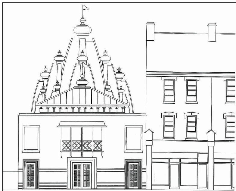
Figure 104: Elevation of mandir to King Street, as designed by Suresh Patel. The sikharas have not been developed to this extent
