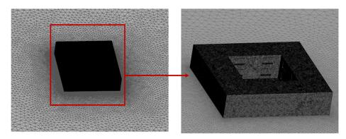
Figure 8. Meshed surfaces of the courtyard and its surrounding microclimate.
