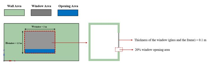
Figure 5. The dimension of each window and the opening area.
