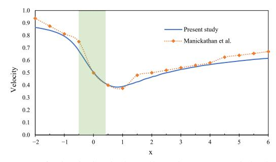
**Figure 14.** Comparison of wind speed on the analysis line, in addition to the vegetation zone under the indication of the green patch in the range of -0.5 to 0.5 on the *x*-axis. (Reprinted with permission from [29]. Copyright 2019 Mohammadi Murtaza and John Kaiser Calautit.).
