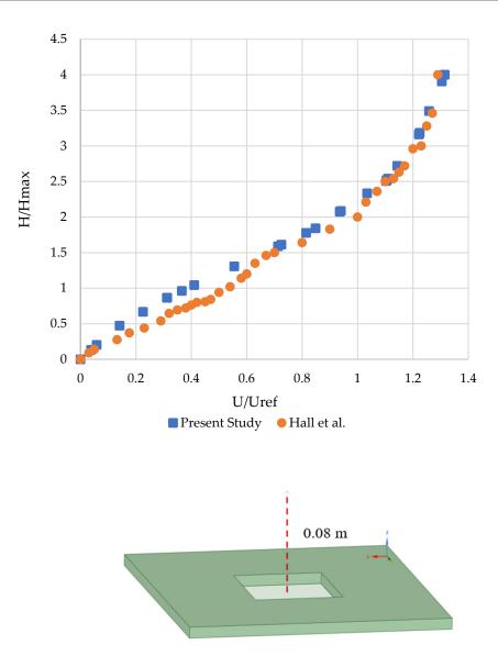
**Figure 11.** Comparison of dimensionless wind velocity along the analysis line (H: height above the ground, Hmax: reference height for the wind velocity, U: wind velocity, Uref: wind velocity at the height of Hmax [27]).
