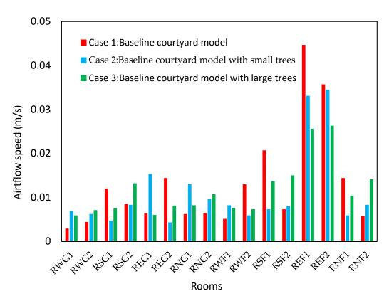
Figure 29. Comparison of wind speed magnitude for Case 1, Case 2 and Case 3 in each room.
