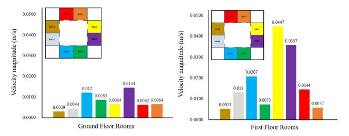
Figure 15. Average wind speed magnitude (m/s) in each room for the baseline courtyard model.
