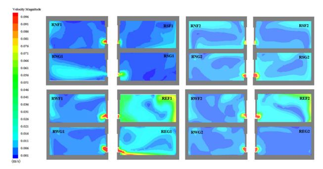
Figure 21. Contours of the wind speed in each room for the baseline courtyard model with four small trees.
