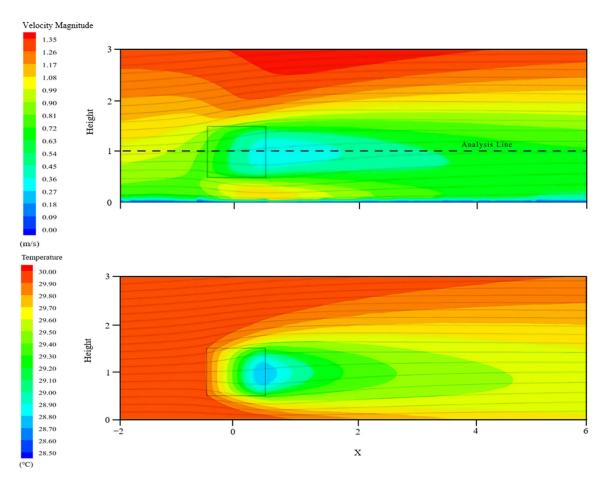
**Figure 13.** Contours of velocity and temperature near the vegetation (black square) based on the validation model. (Reprinted with permission from [29]. Copyright 2019 Mohammadi Murtaza and John Kaiser Calautit.).
