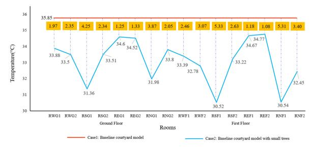
Figure 19. Comparison of air temperature for Case 1 and Case 2 in each room.
