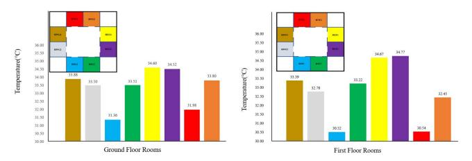
Figure 17. Average air temperature (°C) in each room for the baseline courtyard model with four small trees.
