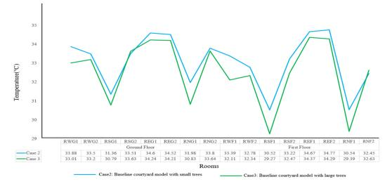
Figure 26. Comparison of air temperature for Case 2 and Case 3 in each room.
