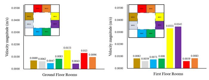
Figure 20. Average wind speed magnitude (m/s) in each room for the baseline courtyard model with four small trees.
