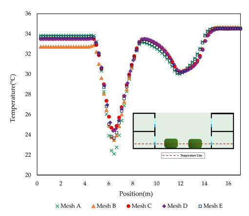
**Figure 9.** Simulated results of temperature along a horizontal center line of the courtyard model with small trees at the height of 0.7 m for the grid sensitivity analysis.
