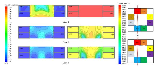
**Figure 30.** Contours for the wind speed magnitude and temperature within the courtyard with small and large trees (S1: X = 7500 mm).
