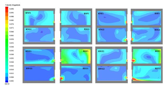
Figure 16. Contours of the wind speed in each room for the baseline courtyard model.
