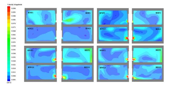
Figure 28. Contours of the wind speed in each room for the baseline courtyard model with four small trees.
