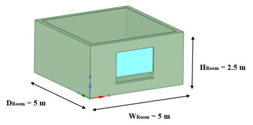
Figure 4. The dimension of each room, naturally ventilated by a window facing the courtyard.
