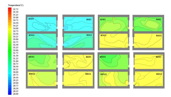
**Figure 24.** Simulated results of the air temperature contour with isotherm in each room for the baseline courtyard model with four large trees.
