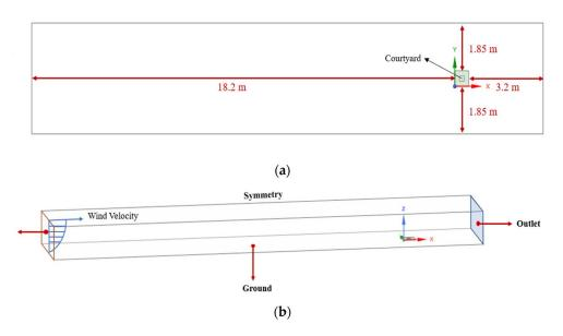
Figure 10. (a) Simulation domain of the validation model. (b) The dimension of the validation model.
