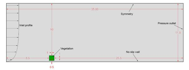
**Figure 12.** Simulation field of the validation model, based on the porous vegetation according to the indication of the green square and centred on the *x*-axis. (Reprinted with permission from [29]. Copyright 2019 Mohammadi Murtaza and John Kaiser Calautit.).
