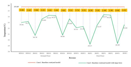
Figure 25. Comparison of air temperature for Case 1 and Case 3 in each room.
