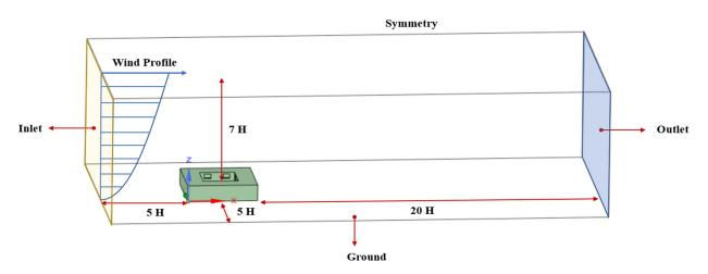
Figure 6. The dimension of the domain and the direction of the wind.
