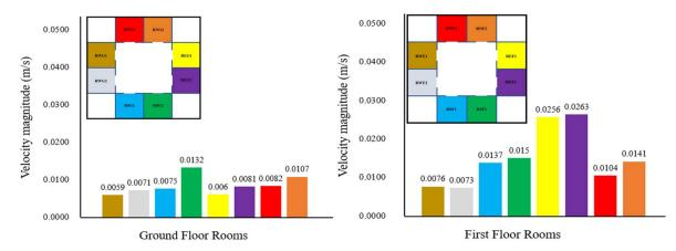
Figure 27. Average wind speed magnitude (m/s) in each room for the baseline courtyard model with four large trees.
