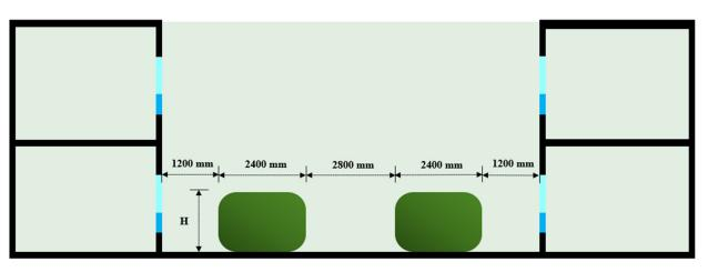
Figure 7. The dimension of the vegetation inside the courtyard model.
