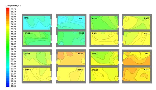
**Figure 18.** Simulated results of the air temperature contour with isotherm in each room for the baseline courtyard model with four small trees.
