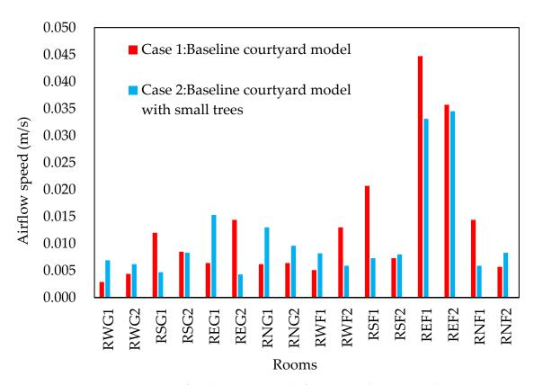
Figure 22. Comparison of wind speed magnitude for Case 1 and Case 2 in each room.
