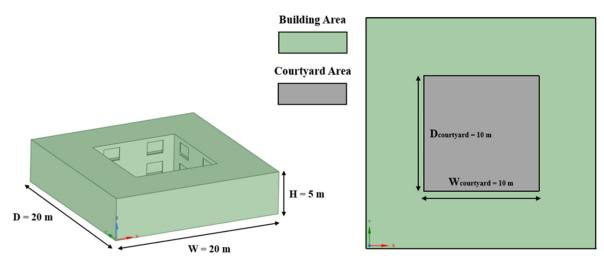
Figure 2. Courtyard model and dimensions.
