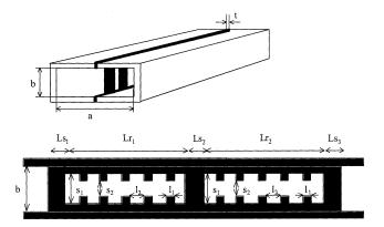
Fig. 1. Layout of the proposed 2 resonator filter.
