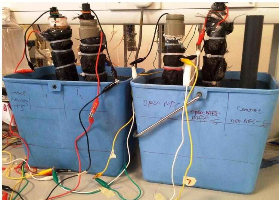
**Figure 9.3:** (A) The soil MFC system during start-up for treating a model PAH-contaminated soil
