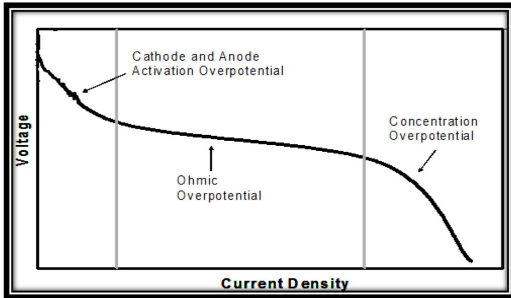
**Figure 1.16:** Regions of a polarisation curve used to assess the MFC performance depicting the energy losses (Image adapted from <http://www.intechopen.com/source/html/16985/media/image17.png>)
