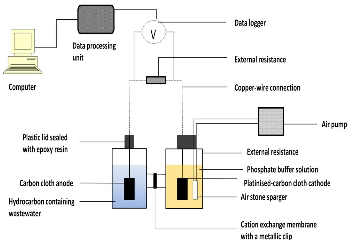
**Figure 2.1:** Schematic diagram of the H-type dual chambered-MFC set-up.
