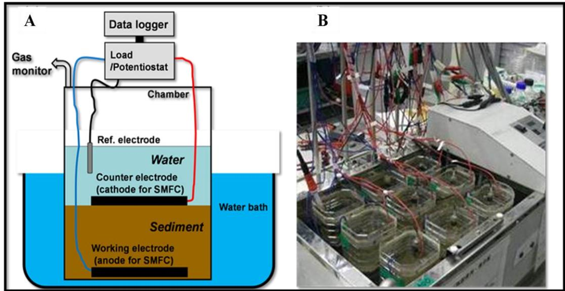
**Figure 1.19:** (A) Schematic diagram of a sediment-type MFC and (B) the laboratory-based sediment MFC set-up (Ueno and Kitajima, 2014).
