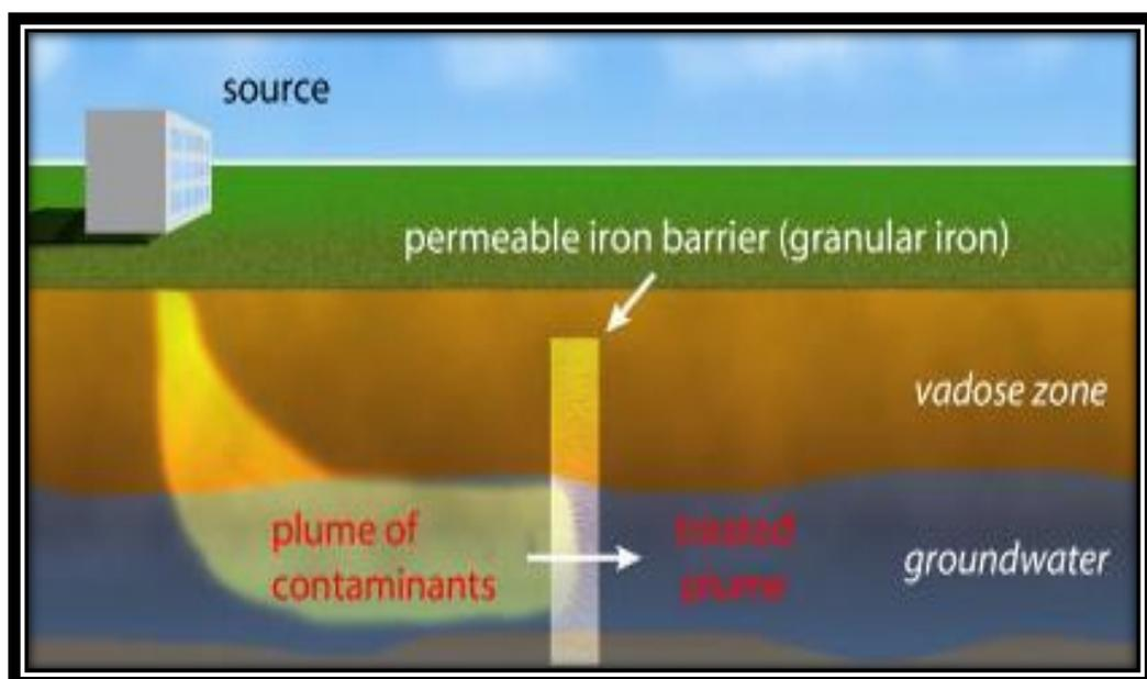
**Figure 1.12:** A typical conceptual design of a permeable reactive barrier (PRB) technology. (Source- [https://commons.wikimedia.org/wiki/File:Iron\\_Wall\\_PRB.jpg](https://commons.wikimedia.org/wiki/File:Iron_Wall_PRB.jpg)).
