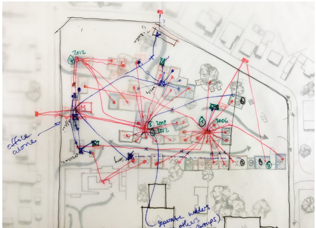
Figure 35: Sketch of the history of electricity distribution at the mall developed in collaboration with traders. Red indicates the current distribution network from five electricity meters that are numbered according to the year of installation (green). Blue indicates the need for new meters that was discussed with traders.
