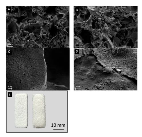
**Figure 1.** SEM images of neat P(3HB) scaffold (**A**), neat P(3HO) scaffolds (**B**), P(3HB)/Cu-doped bioactive glass (BG) composite (**C**), and P(3HO)/Cu-doped BG composite (**D**). (**E**) Digital camera images of P(3HB)/BG (left) and P(3HO)/BG (right) scaffolds.
