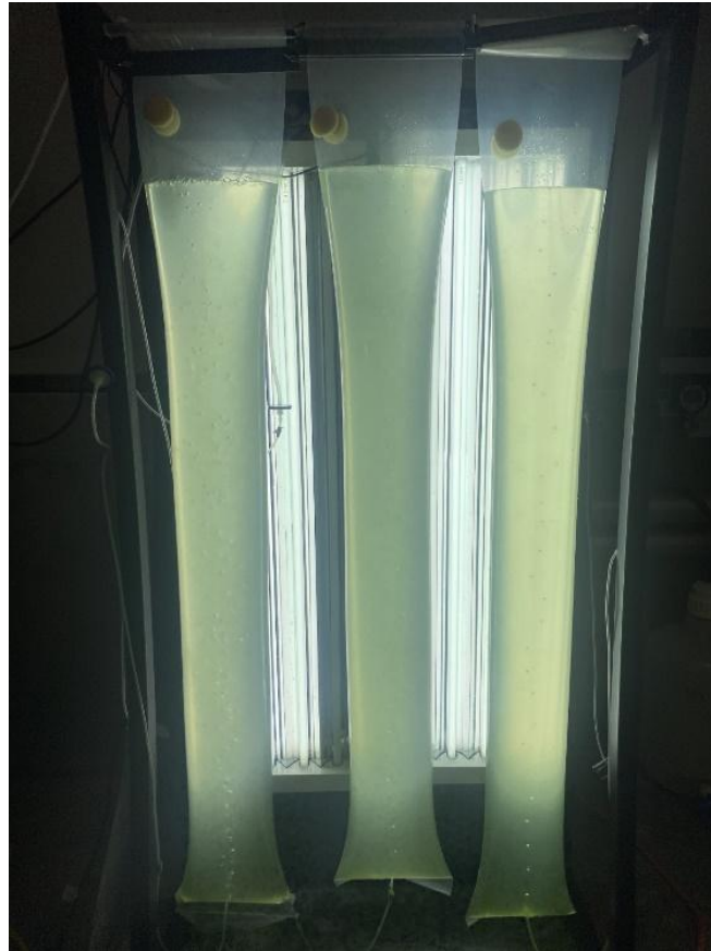
Figure 2.9 The bioreactor in operation.
