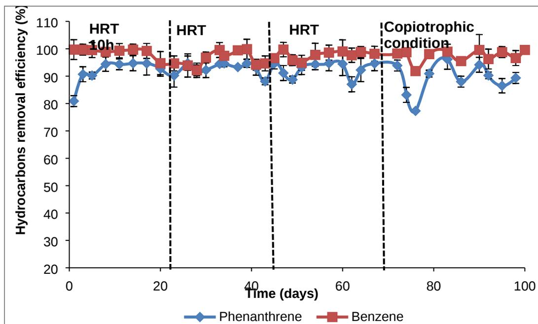
**Fig. 9:** COD removal and Hydrocarbons removal efficiencies at different HRTs and copiotrophic condition at ambient temperatures (15-25°C) using adapted microbial consortia. Error bars  $\pm$  SD are based on duplicate measurements.
