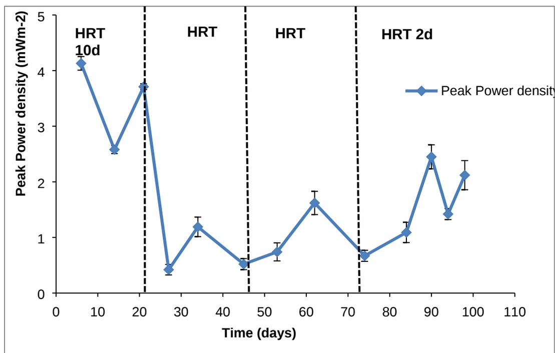
**Fig. 4:** Profile of peak power densities produced at different HRTs in a tubular MFC over 100 days continuous operation at ambient temperatures (10-25 °C) using adapted microbial consortia. Values are means of duplicate experiments  $\pm$  SD.
