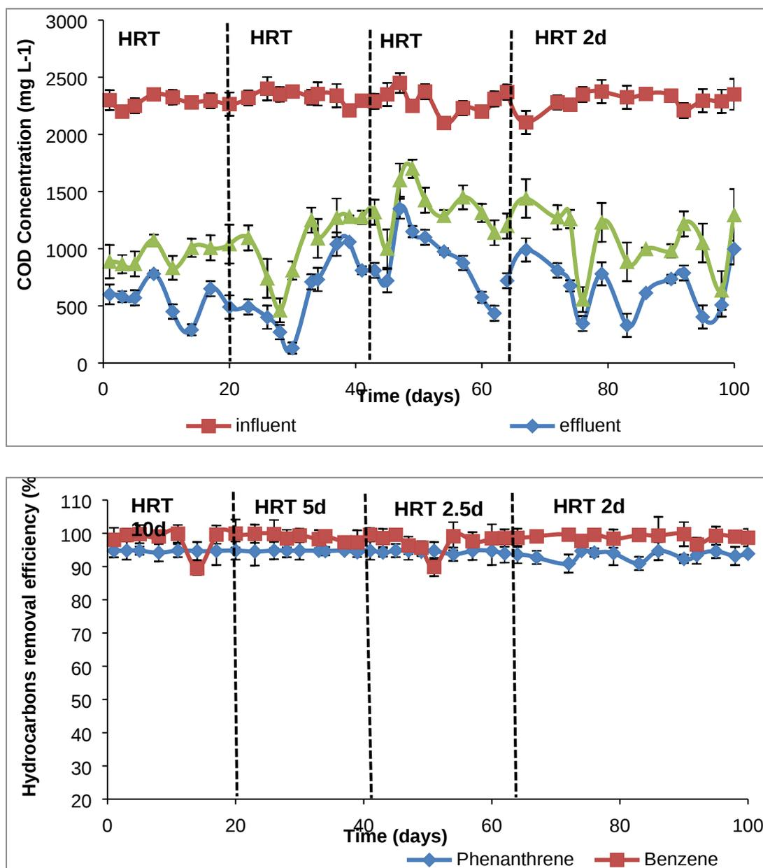
**Fig. 3:** (A) COD removal and (B) Hydrocarbons removal efficiencies at various HRT regimes over a period of 110 days of continuous MFC operation at ambient temperatures (14-25 °C) using adapted microbial consortia. Values are means of duplicate experiments  $\pm$  SD.
