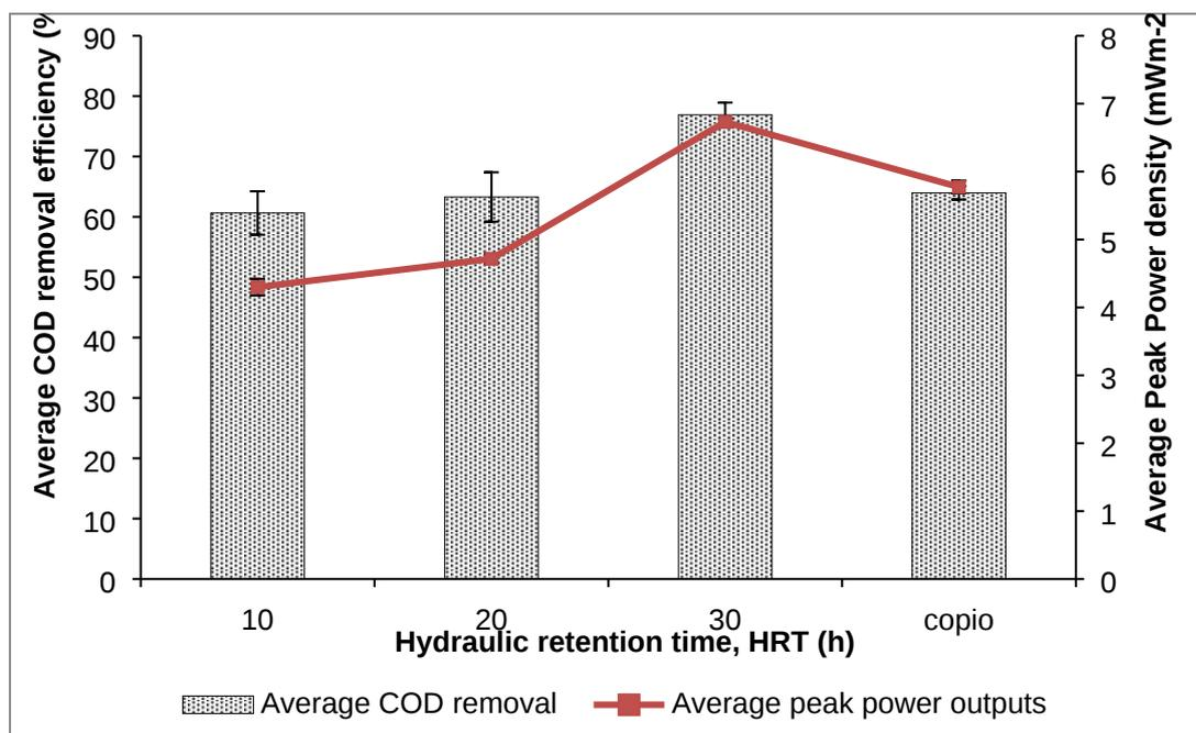
**Fig. 10:** Average COD removal efficiencies and peak power densities generated as a function of time at different treatment conditions in a novel tubular MFC system over 100 days period of continuous operation.
