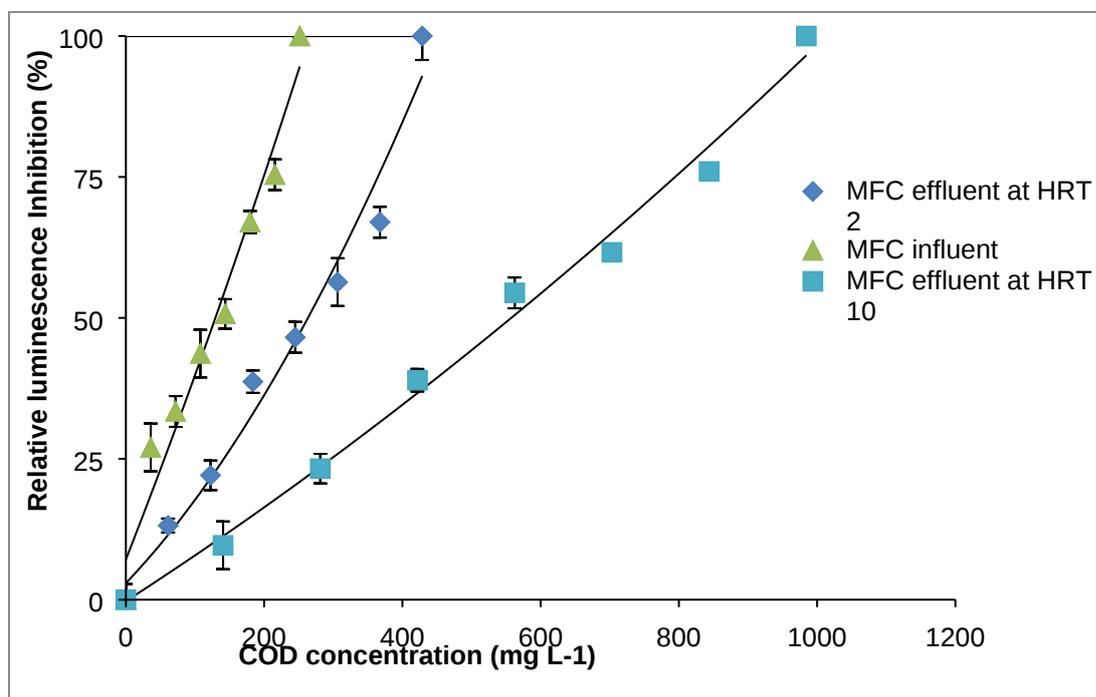
**Fig. 8:** Bioluminescence based toxicity determinations of MFC effluent and influent at HRTs 10 and 2 days using bioluminescent marine bacteria, *V.fischeri*. Values are means of duplicate experiments  $\pm$  SD.
