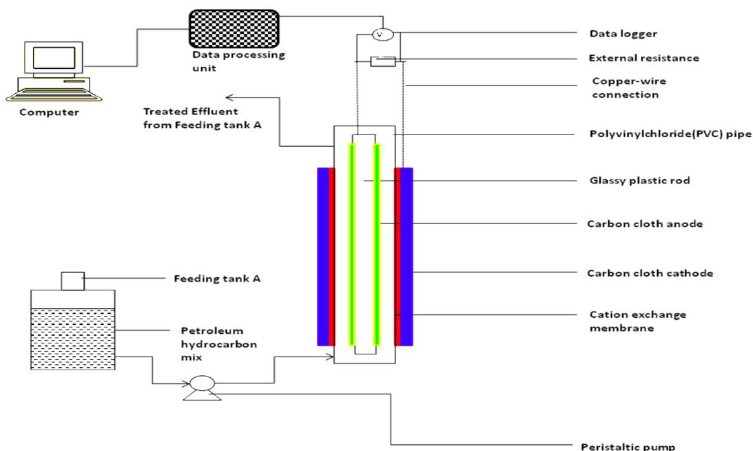
**Fig. 2:** Schematic diagram of the tubular MFC reactor in an up-flow configuration used for the treatment of petroleum hydrocarbon containing synthetic wastewater for a possible *ex situ* application.
