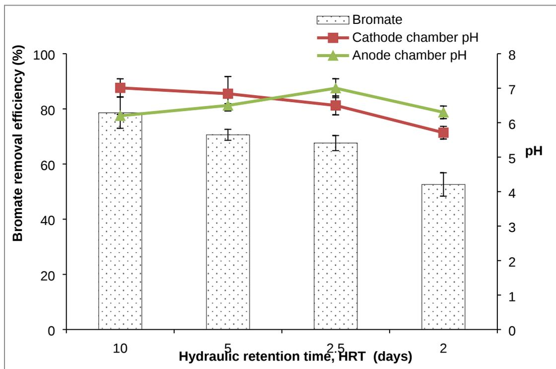
**Fig. 6:** Bromate removal performances and changes in pH in the novel tubular MFC reactor over 110 days operation at ambient temperatures (10-25°C) using adapted microbial consortia. Error bars  $\pm$  SD are based on duplicate measurements.
