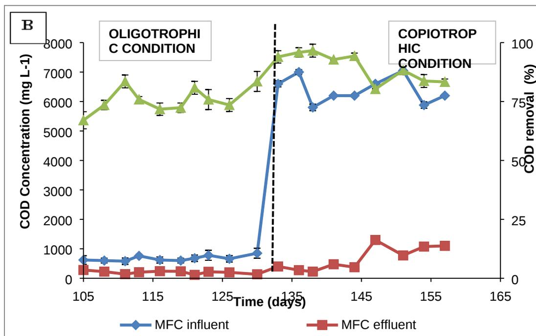
**Fig. 7:** (A) Degradation performance of the tubular MFC at copiotrophic (substrate) conditions (B) COD removal at oligotrophic and copiotrophic (substrate) conditions operated in a continuous mode at HRT of 10 days. Error bars  $\pm$  SD are based on duplicate measurements.
