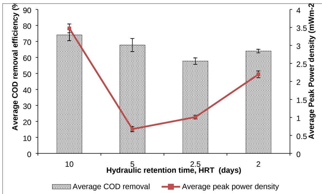
**Fig. 5:** COD % removal and peak power density over the test period in MFCs at different HRTs in the novel tubular MFC at ambient temperatures (10-25 °C) using adapted microbial consortia. Error bars  $\pm$  SD are based on duplicate measurements.
