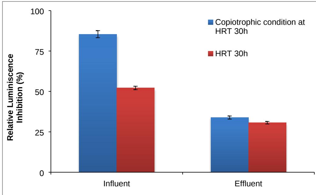
**Fig. 11:** Toxicity levels of MFC effluents at HRT 30 h and copiotrophic condition using adapted microbial consortia as inoculum source. Values are means of duplicate experiments  $\pm$  SD.
