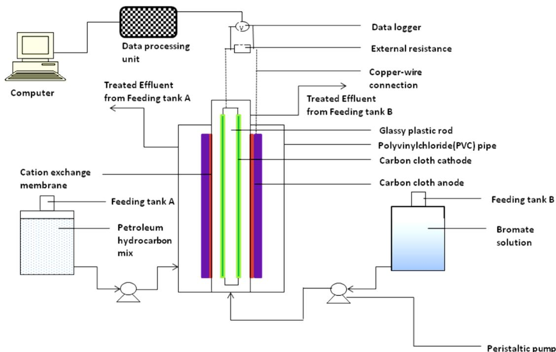
**Fig. 1:** A schematic diagram of the tubular MFC reactor in an up-flow configuration for the treatment of hydrocarbon-containing synthetic wastewater for *in situ* applications.
