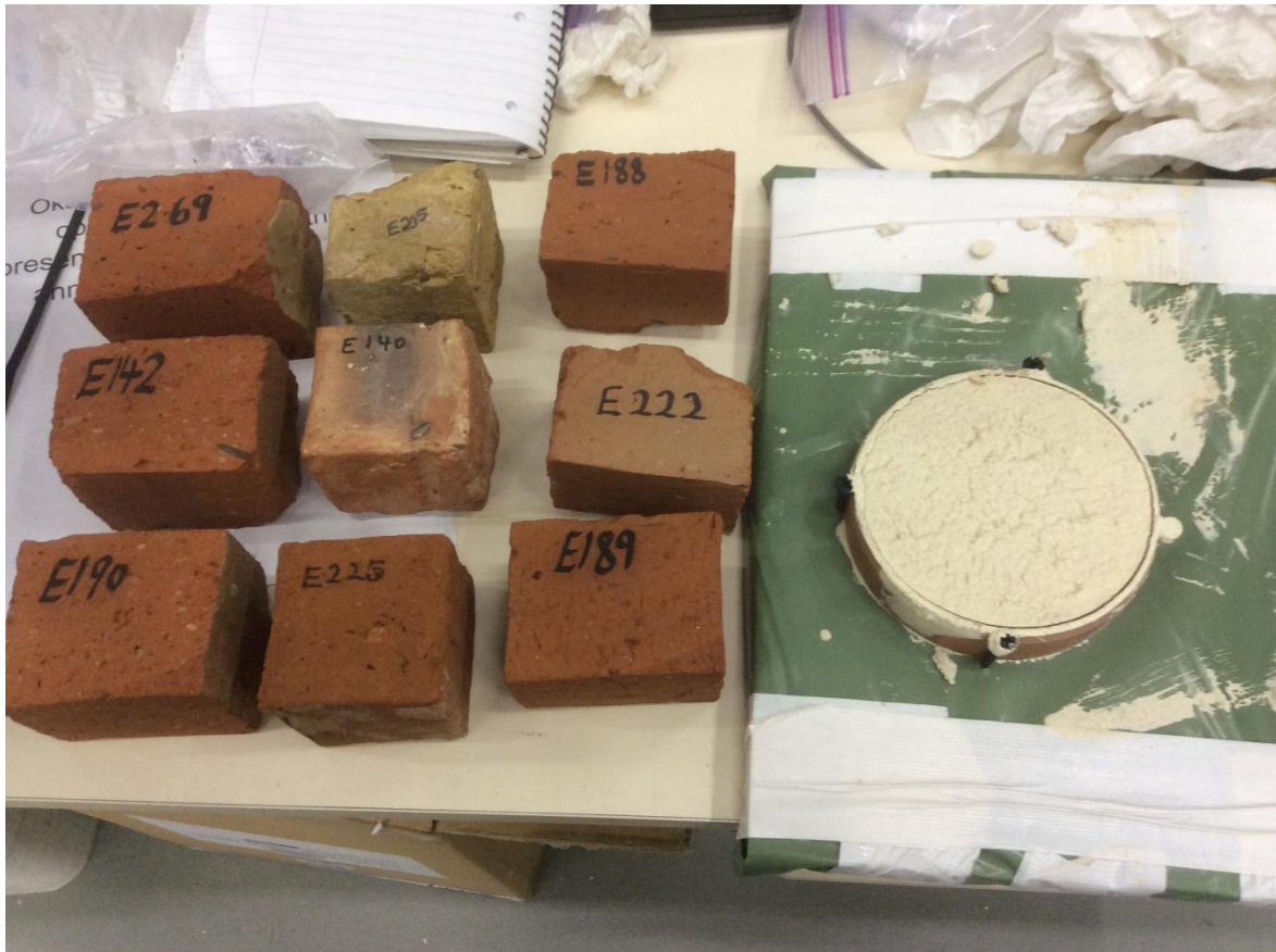
Figure 6: Brick and mortar samples tested for Thermal Conductivity at the National Physical Laboratory.
