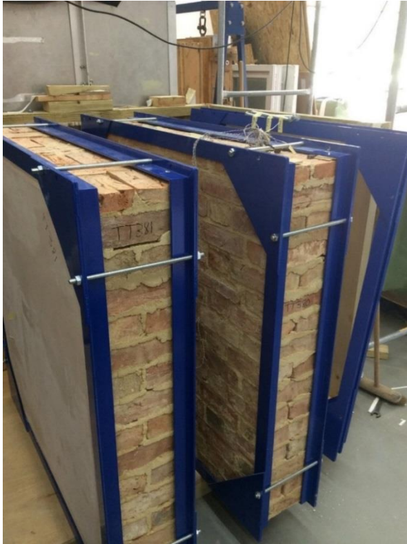
Figure 31: Two of the BRE built walls which are held in place within the specifically designed blue 'moving frames' to allow them to be lifted into the hot-box.
