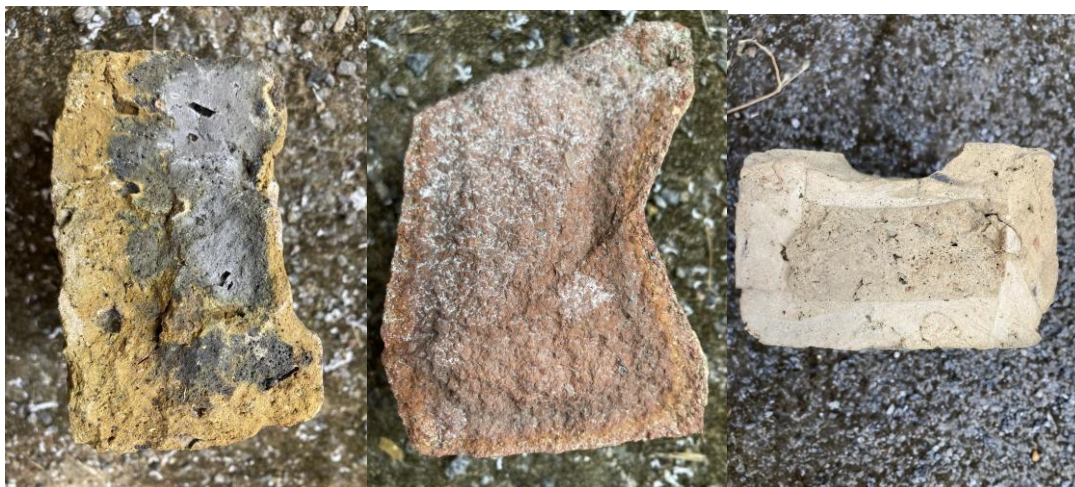
Figure 10: Three sections of bricks from solid wall homes. Left: London stock brick showing internal clinker and other inclusions, gaps and extensive cavities. Centre: Red brick demonstrating concentric discolouration. Right: Stock brick showing significant differences in internal structure and colouration around harder and more uniform margin, likely to indicate incomplete firing.
