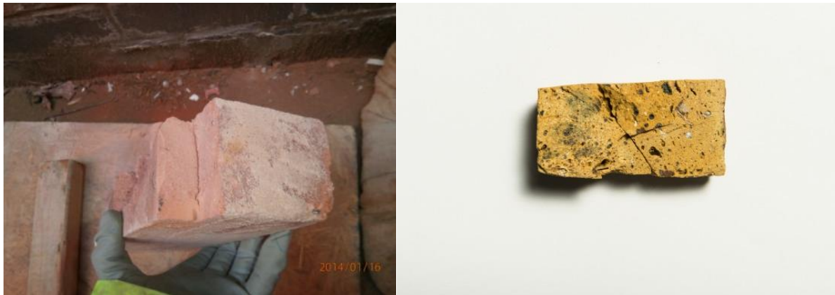
Figures 5 and 6: A brick where a sample has been cut off, and a sample of brick from the back of a removed brick (dimensions of this sample are approximately 30mm x 30mm x 60mm. Larger samples were taken in the second fieldwork period to allow for direct testing of thermal conductivity as described in Section 4).
