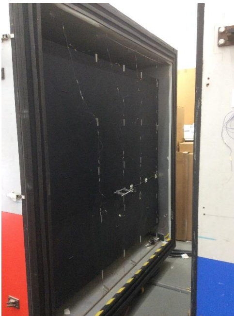
Figure 28, 29 and 30: Photographs of the NPL Wall Hot-Box Apparatus. The hot side of the box, marked in red is on the left hand side of the photographs. The cold side, marked in blue, is on the right hand side.
