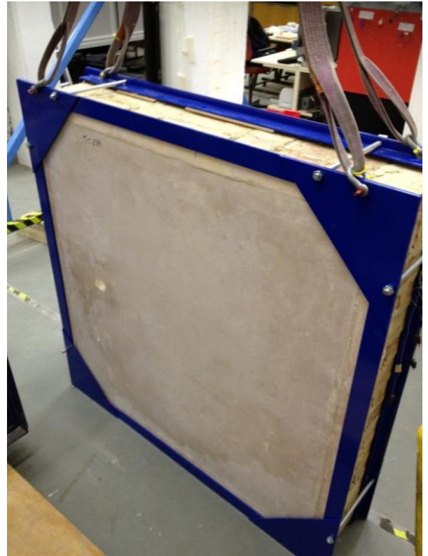
Figure 32: Each wall was plastered with a gypsum 'hardwall' plaster. This is a modern plaster, as it is our assumption that many ancient plasters will have been replaced.
