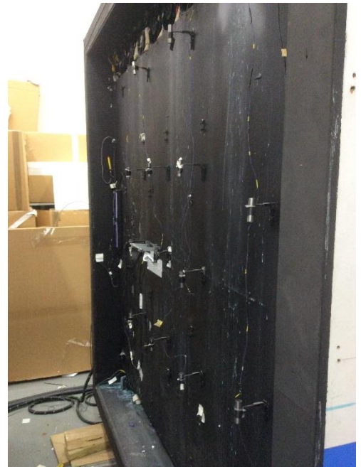
Figure 28, 29 and 30: Photographs of the NPL Wall Hot-Box Apparatus. The hot side of the box, marked in red is on the left hand side of the photographs. The cold side, marked in blue, is on the right hand side.
