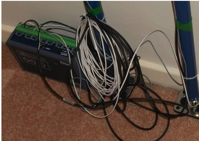
Figure 3: An Eltek 851L datalogger, recording EMF and thermistor readings from the sensing equipment
