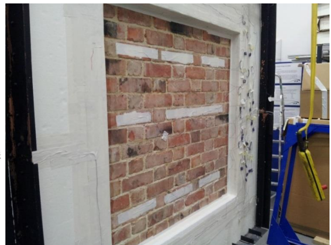
Figure 42: A completed wall, within the EPS guarding, ready to be placed into the hot-box. Once in this position the wall could be rolled into place on castors.
