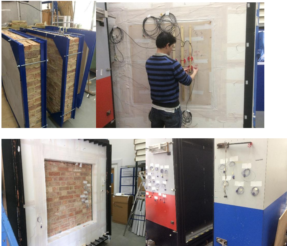
Figure 2: The NPL hot-box experiments in Report 2. From upper left. (1) Two sections of solid wall inside testing frames. (2) Me installing heat flow meters on the plastered (warm side) of the wall to allow direct comparison with hot box measurements (3) The external (cold side) of a wall, surrounded by insulant to minimise heat losses (4) A view of the open hot box. Warm side coloured red, cold side coloured blue. Various thermocouples used in monitoring test are attached to the apparatus.
