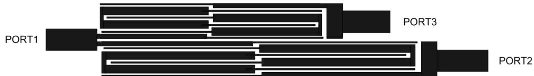
Fig. 4. Layout of proposed microstrip three-port multiplexer
