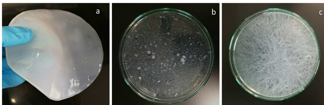
Figure 6.1 Production of cellulose fibres through mechanical grinding: a) bacterial cellulose pellicle, b) cellulose after grinding with normal blender, c) cellulose after homogenisation with immersion hand blender.
