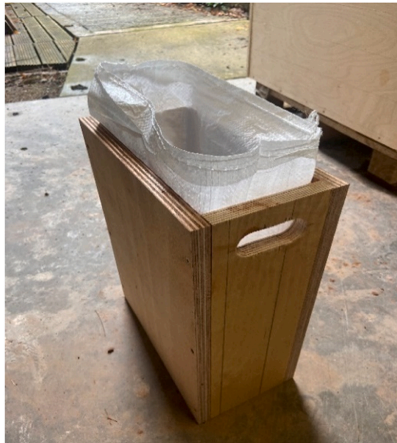
Fig. A. 1. Earthbag block mould.
