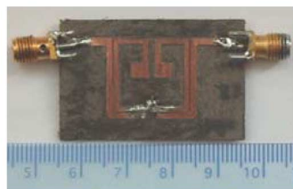
Fig. 7. (a) Measured and Simulated Response; (b) photograph of fabricated filter.
