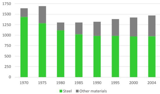
**Figure 26: Weight of an average US car (kg) and its steel content. Source: U.S. Geological Survey (2006).**
