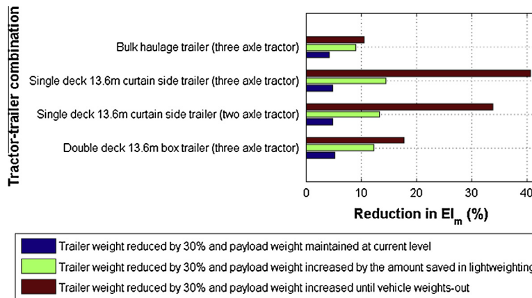
Fig. 9. Estimates of energy consumption reductions that can be achieved through three scenarios involving lightweighting. Note that the third scenario, which involves reducing trailer weight by 30% and increasing the payload until the vehicle reaches its maximum legal GVW (weights-out), will be difficult to achieve for single deck trailers used in grocery distribution because of their volume restrictions. However, this scenario should be achievable in bulk haulage trailers and double-deck trailers used in grocery distribution.
