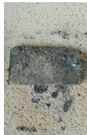
Fig. 56, 57, & 58. Smelting silicon powder mixed with boron oxide at over 1410°C in a treated pizza oven brick, ceramic insulation, microwave oven, to produce silicon flakes. CW, London, 2012.
