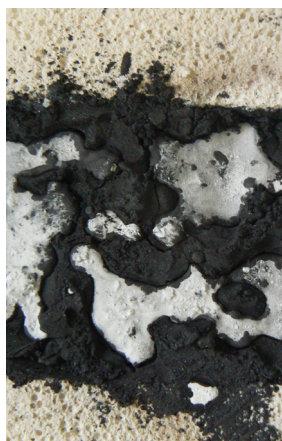
Fig. 56, 57, & 58. Smelting silicon powder mixed with boron oxide at over 1410°C in a treated pizza oven brick, ceramic insulation, microwave oven, to produce silicon flakes. CW, London, 2012.
