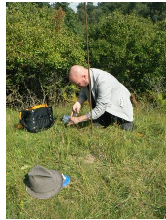
Fig. 32. Placing computer mineral mix under a lightning conducting rod for the creation of custom fulgurites, Grimes Graves, 2011.
