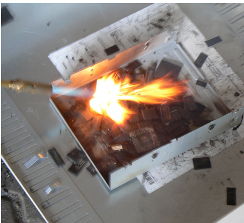
Fig. 21, 22, & 23 Day Two: Heating crushed ICs; preparing Aqua Regia: over excitable Aqua Regia and crushed ICs after heating.
