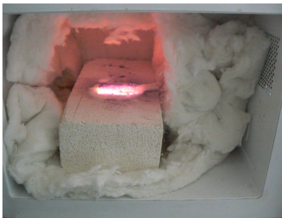
Fig. 56, 57, & 58. Smelting silicon powder mixed with boron oxide at over 1410°C in a treated pizza oven brick, ceramic insulation, microwave oven, to produce silicon flakes. CW, London, 2012.
