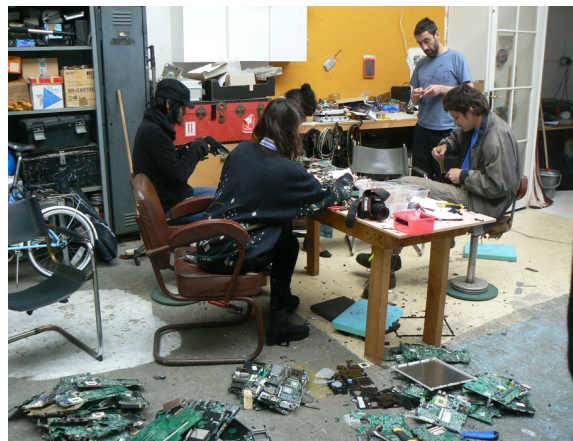
Fig. 3. Day One: One location for the removal of selected parts from junk motherboards.
