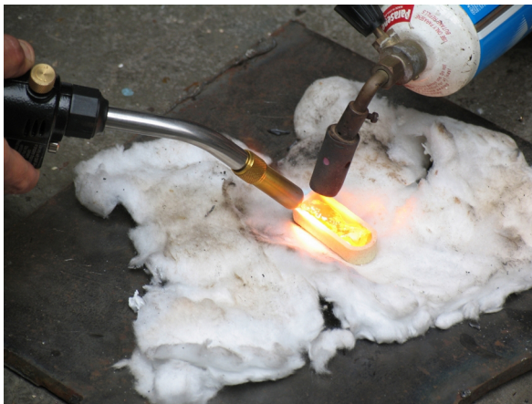
Fig. 10. Day Two: Using gas torches to melt recovered copper to make crude cuprous oxide semi-conductors.
