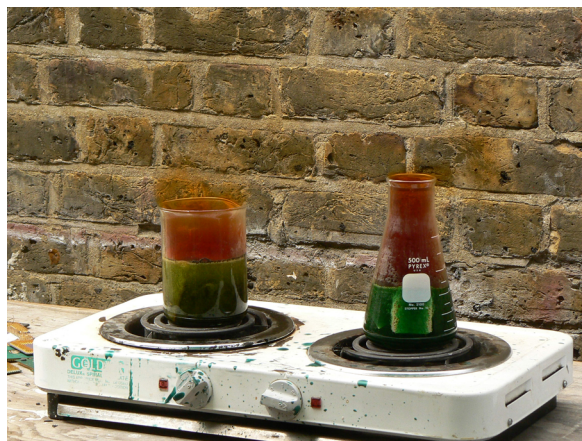
Fig. 5. Day One: Heating the Aqua Regia and crushed processors to accelerate the dissolution of gold and other base metals.
