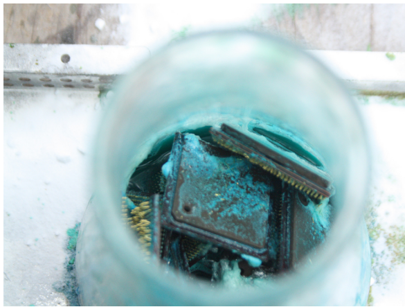
Fig. 8. Day Two: Using nitric acid to leach base metals including silver from processors.
