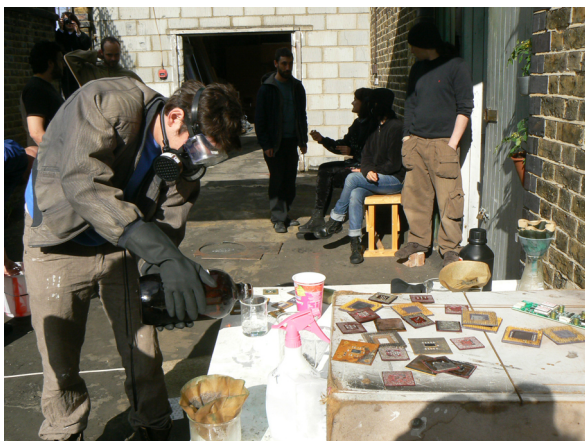
Fig. 4. Day One: Adding nitric acid to crushed integrated circuits for dissolution of silver and copper.
