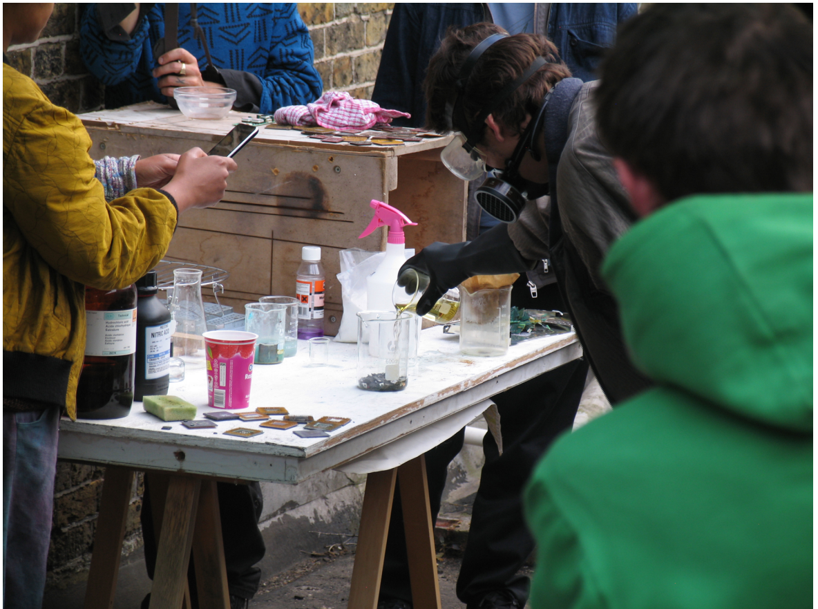
Fig. 1. Decrystallisation Workshop, London, May 2011: Preparation of Aqua Regia (nitric/hydrochloric acid mix) being added to crushed processors to make a gold solute as a stage on the way to attempt to recover gold metal.
