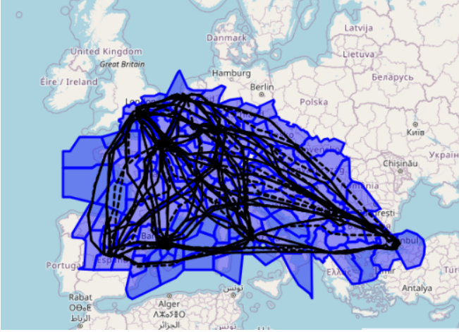
Figure 3. Depiction of the scenario used to run the model. Blue shapes represent sectors, solid black lines are 'routes A' and dotted black lines are 'routes B'.
