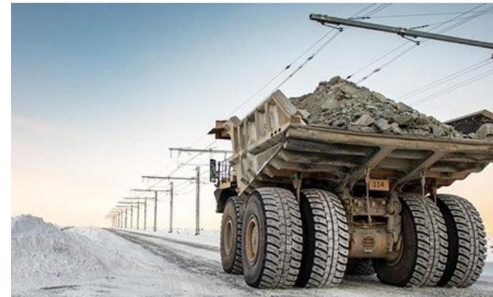
CAT Trolley Assist: diesel –electric overhead catenary mining trucks
