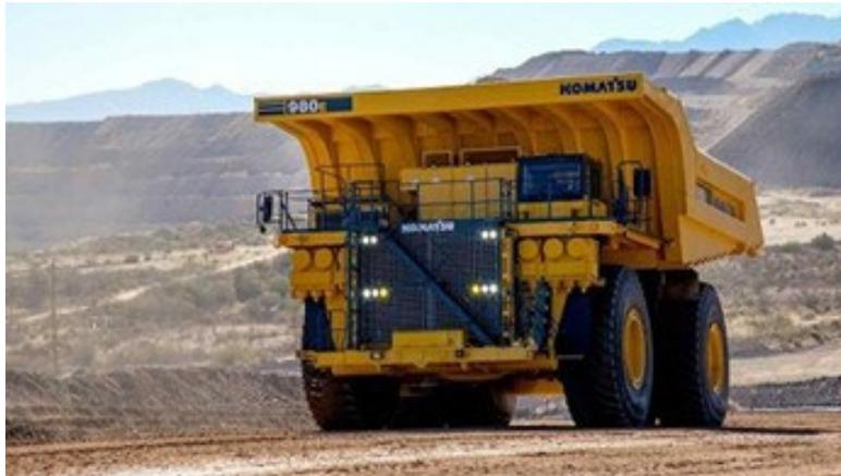
Komatsu: hydrogen fuel cell powered dump truck
