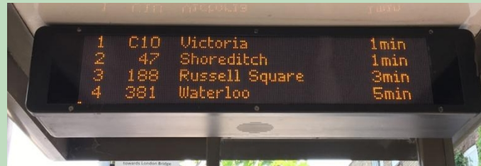
Figure 4. RTI display panel at Bermondsey Station Bus Stop A (Source: Authors)
