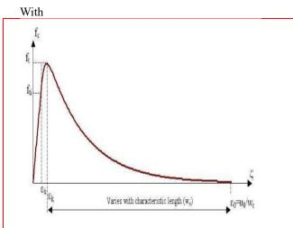
Fig. 8 Damage evaluation function (softening curve) LUSAS, 2016)
