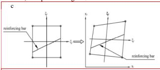
Fig. 7 Embedded reinforcing bar element in the local and global system
