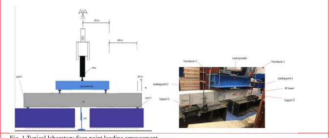
Fig. 1 Typical laboratory four-point loading arrangement
