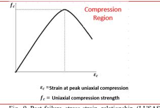
Fig. 9 Post-failure stress-strain relationship (LUSAS, 2016)
