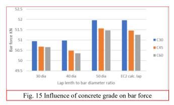
Figure 15 shows the effect of concrete on the lapped bar force. Figure 14(a) shows the inverse relationship between the concrete grade and the lapped bar force; an increase in zero shear distance results in a decrease in the lapped bar force.
