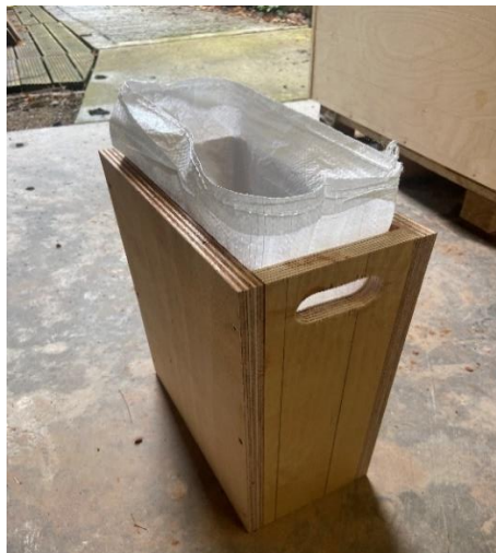
Fig. A. 1 Earthbag block mould
