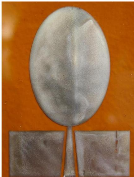
**Figure 4.5–2: Photograph of the fabricated inkjet-printed antenna.**
