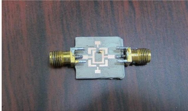
Figure 3.4–3: Photograph of the fabricated PCB filter.
