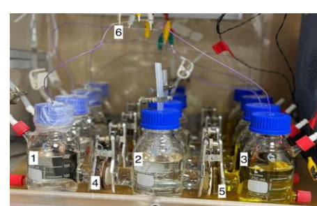
Figure 3 – The MDC Photo-bioreactor used in the experiment – 1. Anode chamber containing synthetic wastewater 2. Desalination chamber containing artificial seawater 3. Cathode chamber containing 1.0M K_3[Fe(CN)_6] 4. AEM 5. CEM and 6. External resistor (20.5 kOhm resistor).
