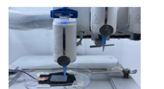
Figure 2 – 3D-bioprinting of S. oneidensis onto carbon electrode surface (bioelectrode) using 3D-bioprinter (XTM, Cellink, Sweden).
