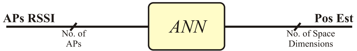
Fig. 4-10 Block scheme of a single ANN position estimation model
