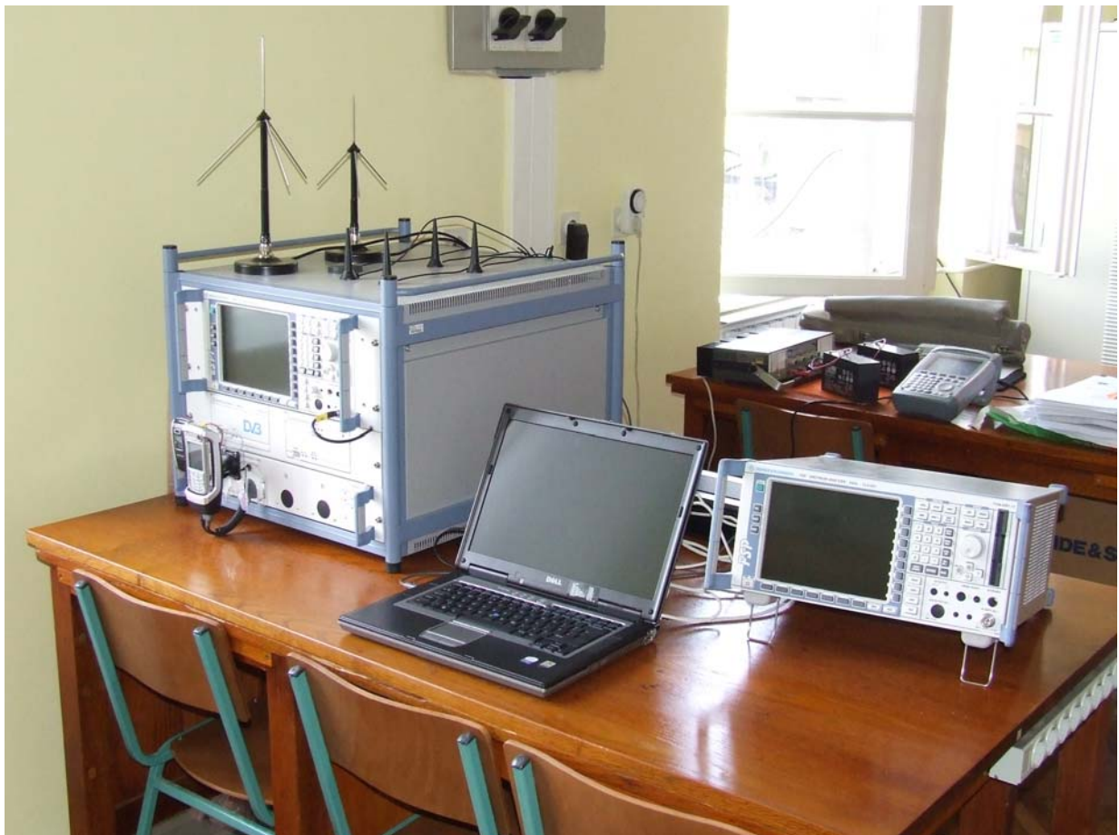
Fig. 5-1 Specialized Measurement System – TMSQ & ROMES (Rohde&Schwarz)
