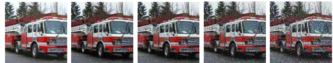
Figure 1: In the presence of noise the recognition of the fire engine deteriorates as Gaussian Noise increases. In the original uncorrupted image (leftmost), top 1% the fire engine is recognized with 66% accuracy. As Gaussian noise is added to the image increasing progressively from standard deviation 0.08 to 0.12, 0.18 and 0.26 (rightmost image), top 1% accuracy for the fire engine is decreased respectively to 60%, 24%, 9% and 0%.
