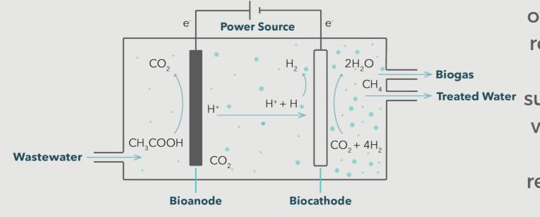
Retention times between 30 and 2.4 days were investigated to align with commercial viability targets. Organic loading rate varied between 0.4 and 6 kgCOD/m³/d. An average COD removal of 93% was observed over the 4 month investigation with on average 83% of the COD being removed in the first two stages of the reactor. A peak stable HRT of 3.1 days was achieved in the primary reactor with 85% COD removal, suggesting that the secondary stage is largely redundant with brewery
