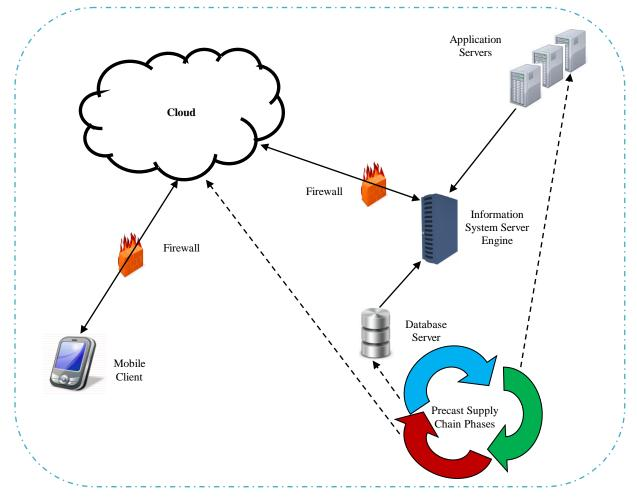
Figure 1: Cloud Computing Information System (CCIS) Architecture for Precast Supply Chain Management
