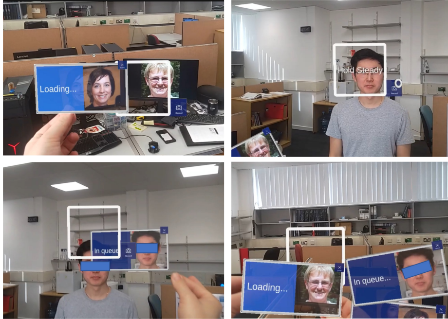
Fig. 4. The automatic recognised faces are uploaded in the queue ready to be analysed by the deep neural network, which provides the skin classification.
