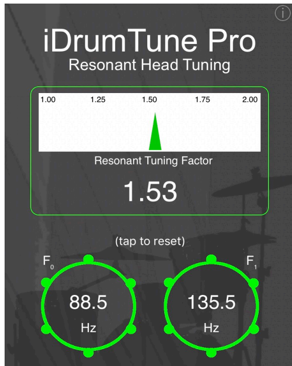
Figure 6. Once f_{01} and f_{11} are recorded, iDrumTune Pro displays the calculated RTF value.
