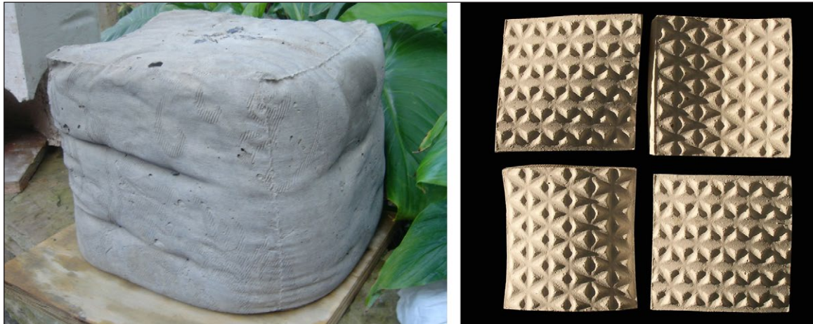
Figure 2: (Left) Concrete cushion fabric formwork experiment. University of Greenwich, UK (Photograph by Jon Goodbun/Cordula Weisser); (Right) Concrete tiles produced through adjustable analogue/digital formwork. Lorin Arnold. Polytechnic Studio, University of Westminster, UK. 2004 (Photograph by Lorin Arnold).
