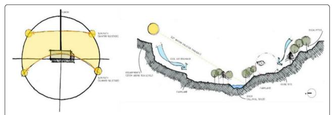
Fig. 1 Left: Orientation as a basic design principle, allows the project to benefit from sunlight and prevailing winds. Right: Site analysis based on Glenn Murcutt's sketches. Heath [8]
