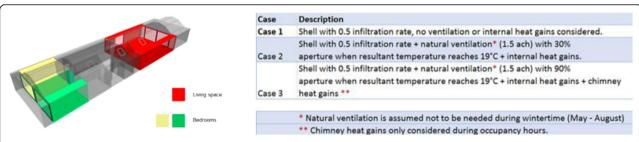
Fig. 17 Left: Thermal assessment and zoning of key spaces in the Ball-Eastaway house. Thermal assessment in EDSL Tas. Right: Summary of thermal cases examined
