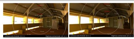
Fig. 23 Luminance (cd/m2) assessment at noon under sunny sky (Equinox) and overcast sky conditions
