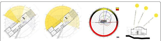
Fig. 13 Left: Ball-Eastaway's orientation vs. sunpath during winter and summer solstice and optimum orientation. Source: NatHERS (2014) Right: Section vs. solar access at noon during summer solstice, equinox and winter solstice
