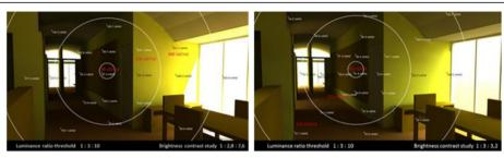
Fig. 16 Luminance (cd/m2) assessment at noon under sunny sky (Equinox) and overcast sky conditions
