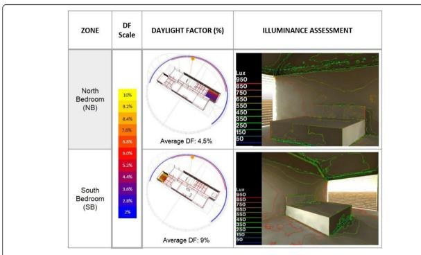
Fig. 8 Daylight performance comparison between bedrooms. Daylight Factor (%) and Illuminance assessment in ECOTECT and Radiance
