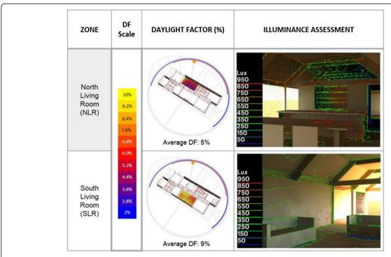
Fig. 7 Daylight performance comparison between living rooms. DF (%) and Illuminance assessment in ECOTECT and Radiance
