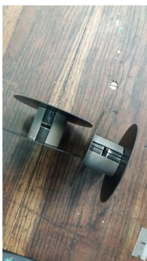
Illustration 4.27: Eyemo rolls, constructed with help of L'Abominable artist film lab in Paris from Bolex 16mm daylight spools enabling me to film during trip
