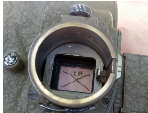
Illustration 3.14: With the lens removed and gate open can mark emulsion with cross to indicates the frame size. Photo Niles Atallah, Dec 2017
