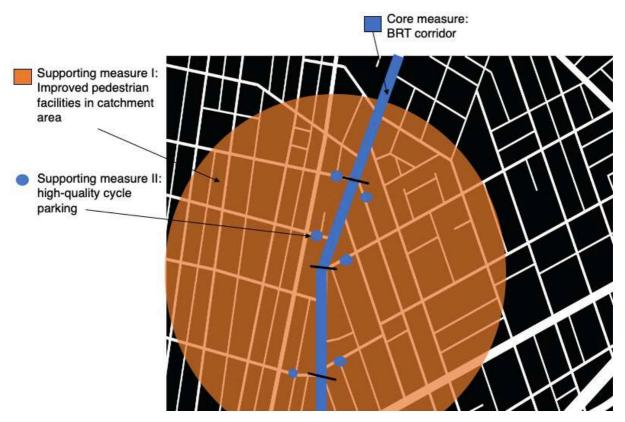
Figure 6.16: Example of spatial clustering of a BRT core measure, and two supporting measures.
