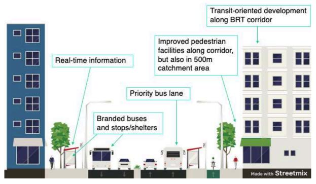
**Figure 6.6:** Illustrative example of 'supporting measures' to enhance the effectiveness of a core measure 'Bus with High Level of Service'.
