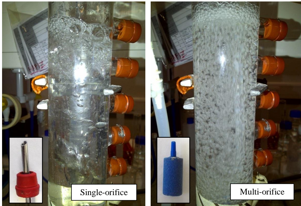
Figure 3. 72: Comparison of bubble sizes created by single and multi-orifice spargers
