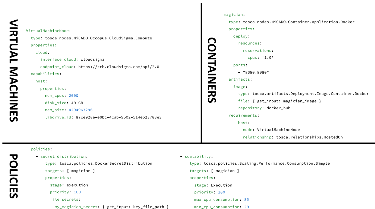
Fig. 9 Application Description Template Instance for Magician
