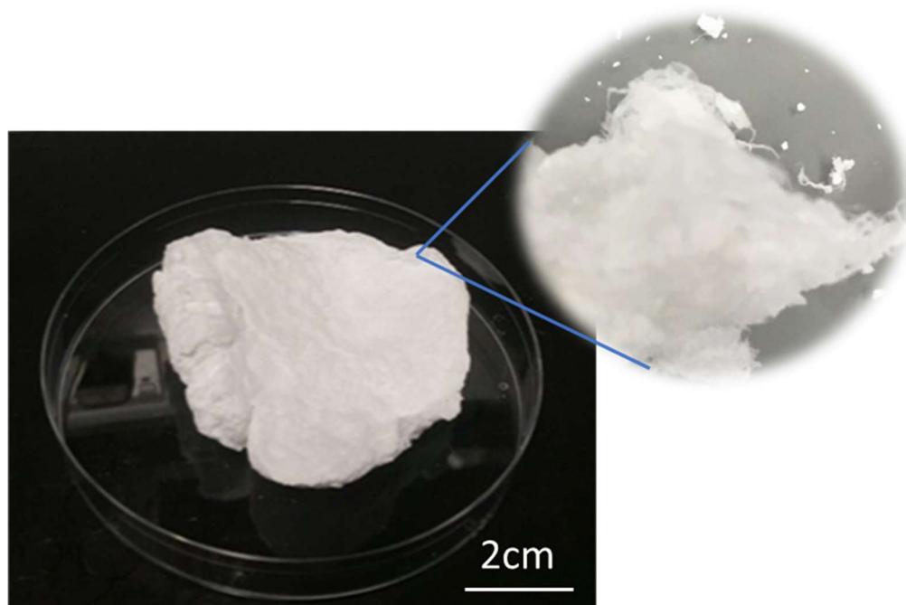
Figure 3.2: Extracted and purified P(3HB) produced by B. subtilis OK2 using glucose as the source of carbon.
