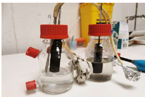
Fig. 1 Graphite rod and Titanium mesh as dual cathode configuration (left). Acetate production in dual cathode and single cathode MESs (right)
