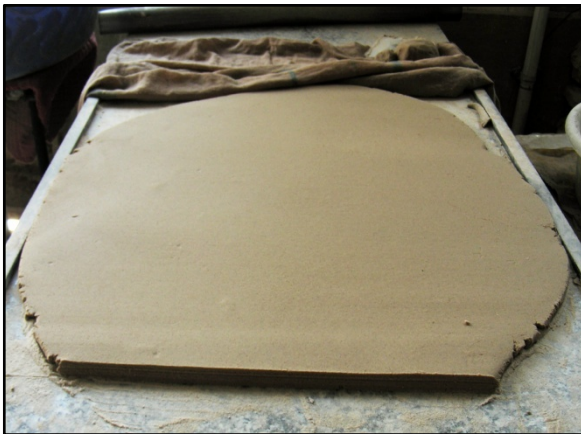
Figure 50: 8 mm thick slab made by rolling the paste with a metal rolling pin between two guiding metal strips
