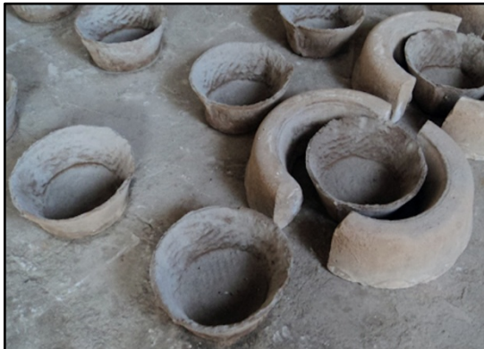
Figure 54: Glazing powder containers are made by pressing slabs of clay into two-parts plaster moulds then left to dry before firing
