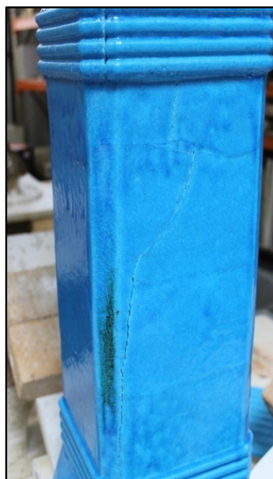
Figure 103: vertical cracks were probably caused by tension in the joints due to various thicknesses in these areas. (Photo by Zahed Tajeddin)
