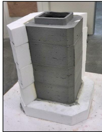
Figure 98: Forming the pillar's sections using the multi-layered mould.(Photo by Zahed Tajeddin)
