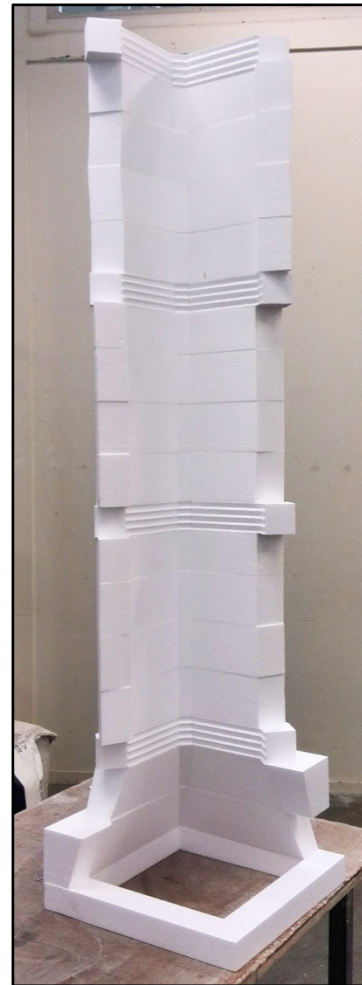
Figure 95: The mould layers for the pillar were cut using the hotwire system. (Photo by Zahed Tajeddin)
