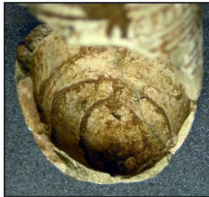
d. The chip showing the coarse sandy core and the thick glaze on the edge
