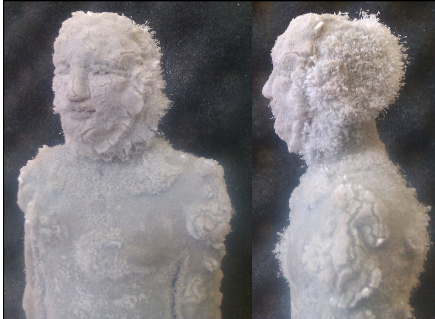
Figure 84: crust and blooms of effloresced sodium salts formed on the surface during drying in an open room with a free flow of air. (Photo by Zahed Tajeddin)
