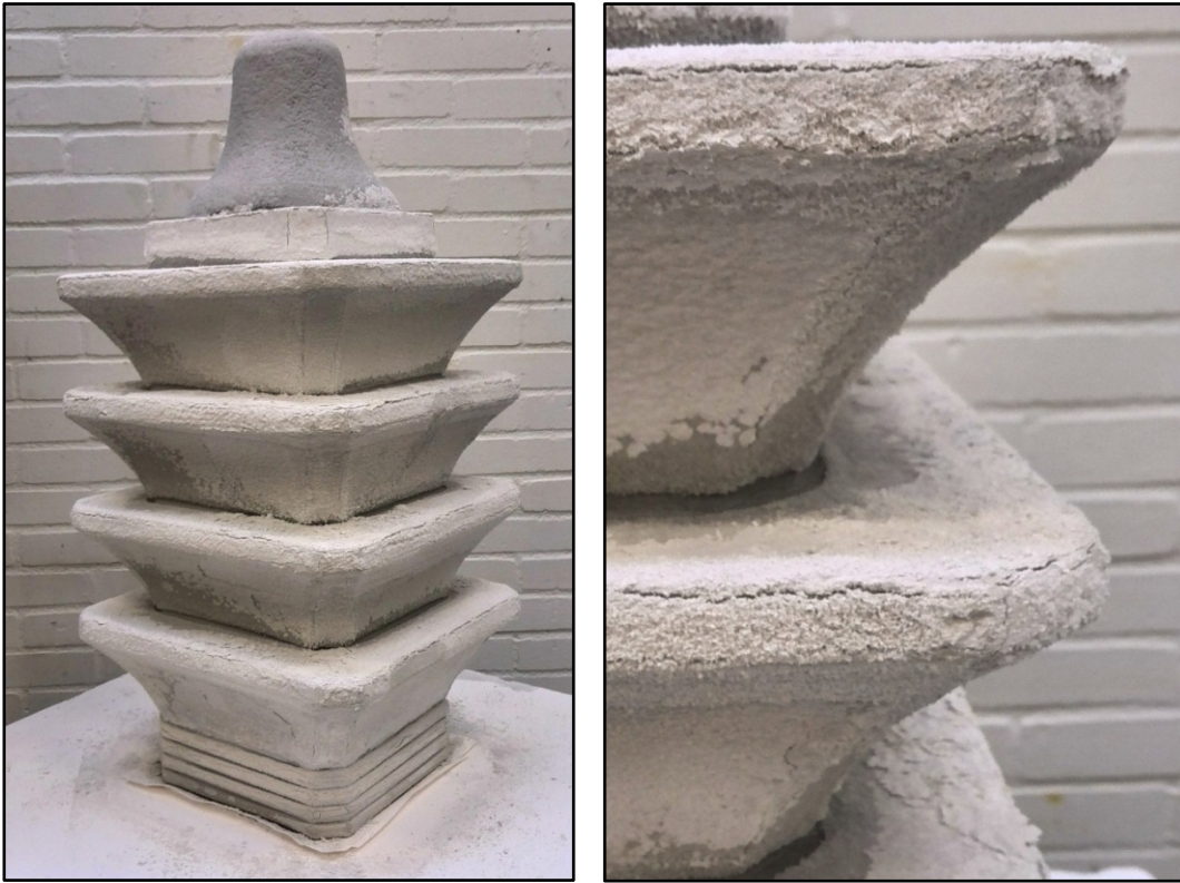
Figure 99: The soda effloresces to the surface upon drying in heated space. (Photo by Zahed Tajeddin)
