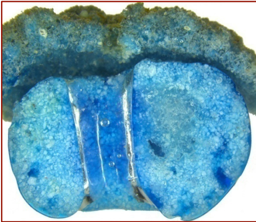
Figure 59: Cross section of a Qom bead and its capsule shows partially fused quartz particles in the bead's body (white colour) surrounded by a continuous glass matrix (blue colour)
