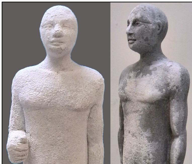
Figure 85: crust of effloresced sodium salts formed on the surface during drying in a 50°C heated chamber. (Photo by Zahed Tajeddin)
