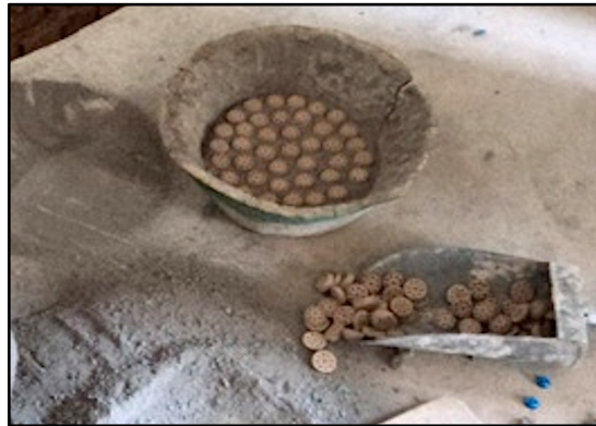
Figure 55: The glazing powder is sprinkled first on the bottom of the container, then alternate layers of beads and powder fill the container to the top
