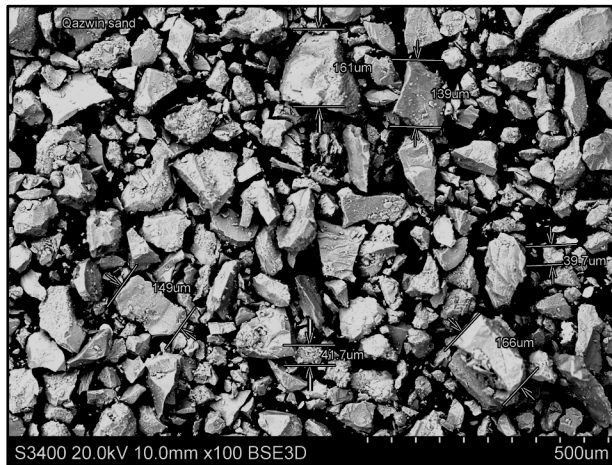
b. Backscattered SEM image of Qazvin quartz in x100 magnification
