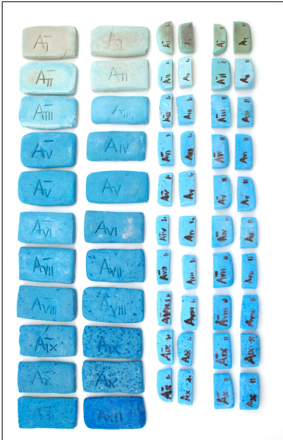
Figure 20: Sets of samples with (50:50) sodium carbonate and bicarbonate ( A^- ), sodium carbonate ( A ) fired to 950°C (left), to 1000°C (middle) and 1100°C (right).
