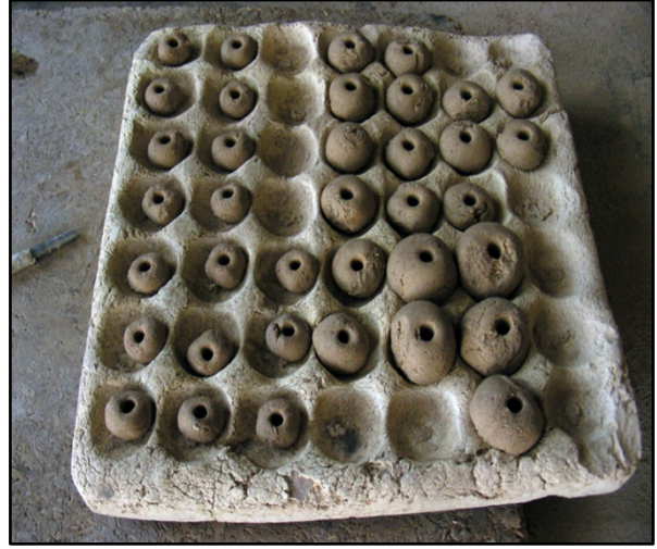
Figure 47: Tray made of fired clay with negative spherical cups to support the shape of the beads while they are pierced with the metal rod (on the left)
