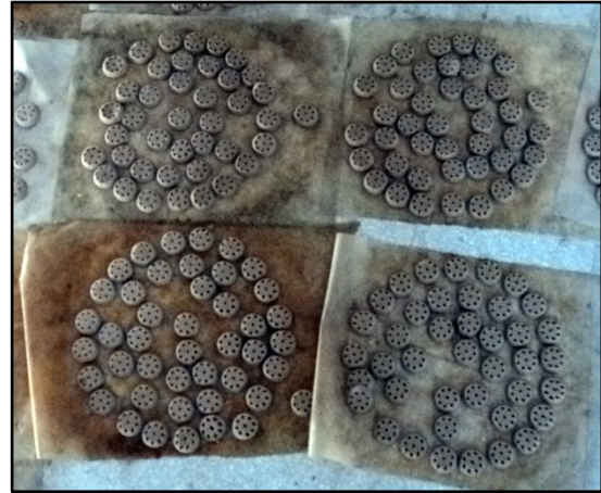
Figure 49: The buttons are tipped over on sheets of paper and left to dry
