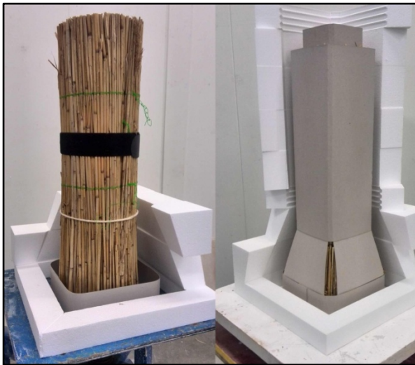
Figure 97: the pillar's sections were built around a core made of cardboard structure filled with canes of reed. (Photo by Zahed Tajeddin)
