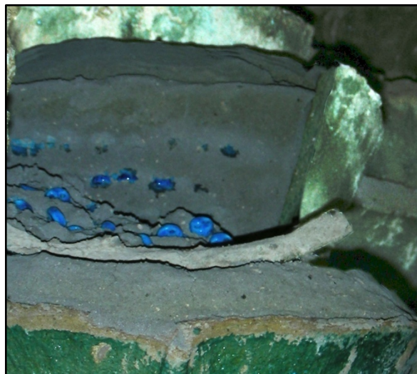
Figure 57: Broken container revealing the beads within the glazing powder
