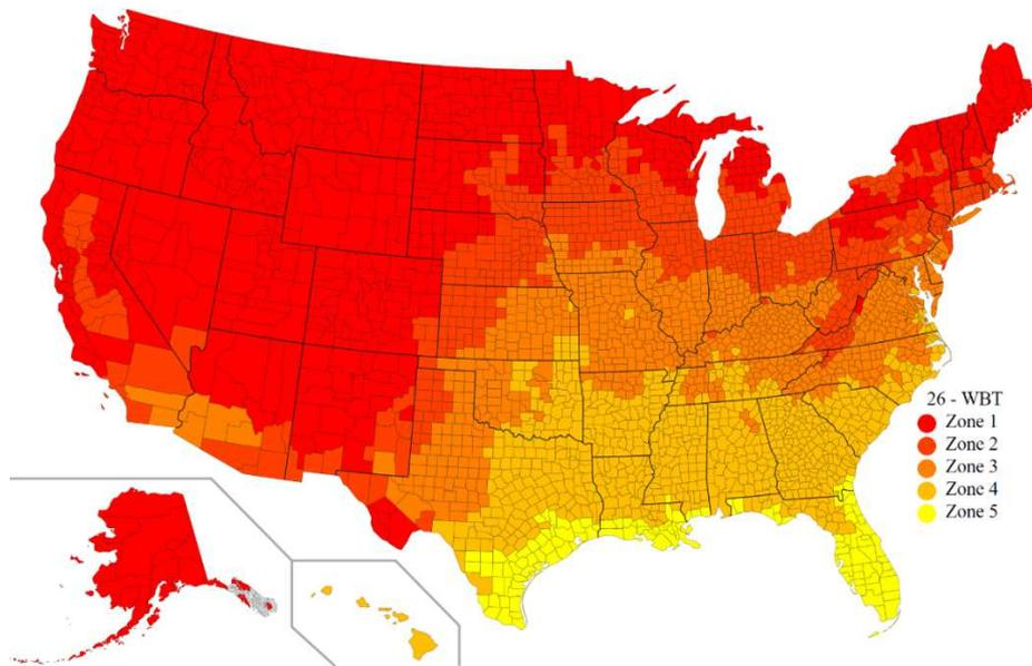
Figure 6 Zones of applicability based on differences between indoor design temperatures and outdoor wet bulb temperatures.
