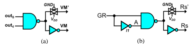
Fig. 7. Possible implementation of circuits generating: (a) VM and VM'; (b) R_s' and R_s .
