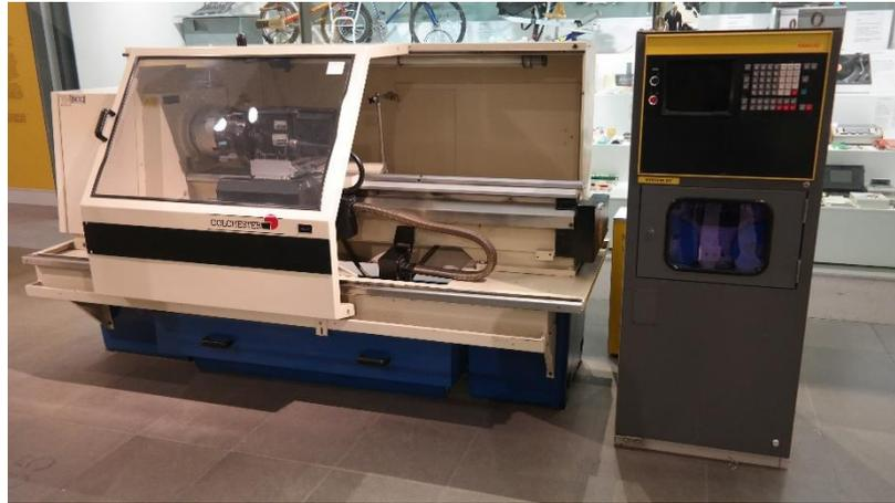
**Figure A.7.** Colchester 200L Lathe and FANUC control system, part of permanent exhibition in the Science Museum, London.
