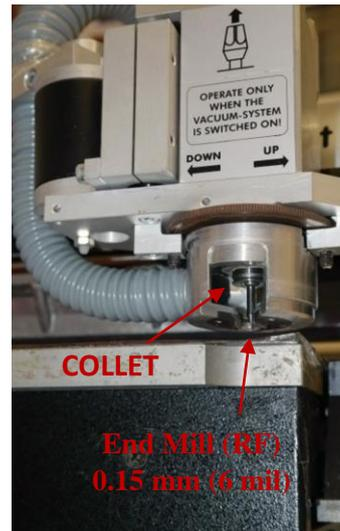
**Figure A.4.** ProtoMat C60 mill/drill head with high-speed spindle having end mill tool in its shaft.
