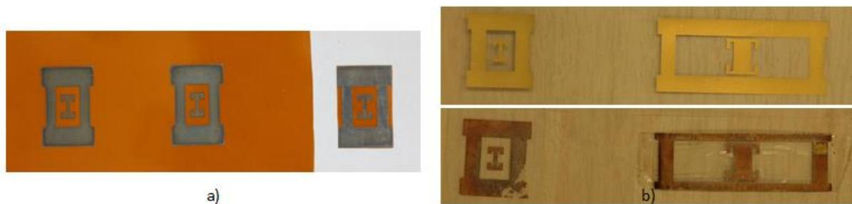
**Figure A.11.** Inkjet-printed E-plane inserts with I-shaped insets for compact waveguide filters: a) Kapton substrate, Dimatix DMP-3000 printer; b) PET substrate, Epson Stylus C88+ printer, without (up) and with (down) copper electroplating.
