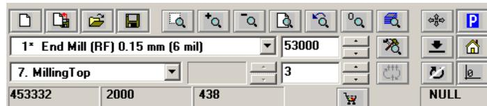
**Figure A.2.** Left section of the BoardMaster Function Bar for selecting current production phase and active tool.
