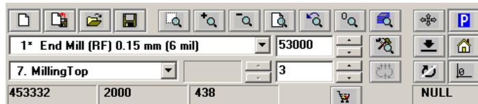
**Figure A.2.** Left section of the BoardMaster Function Bar for selecting current production phase and active tool.
