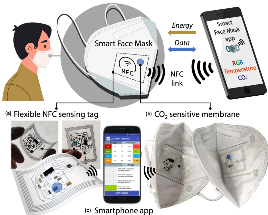
Figure 9. Overview of the NFC-based smart facemask for real-time wireless CO 2 measurement. (a) NFC sensor tag that is flexible. (b) CO 2 sensor membrane on a flexible tag connected to the inside layer of a regular FFP2 facemask. (c) Custom-developed smartphone applications provide power and enable bidirectional communication. Images reused from [226], with no changes. CC-BY 4.0 licence ( https://creativecommons.org/licenses/by/4.0/ ), accessed on 8 October 2023).
