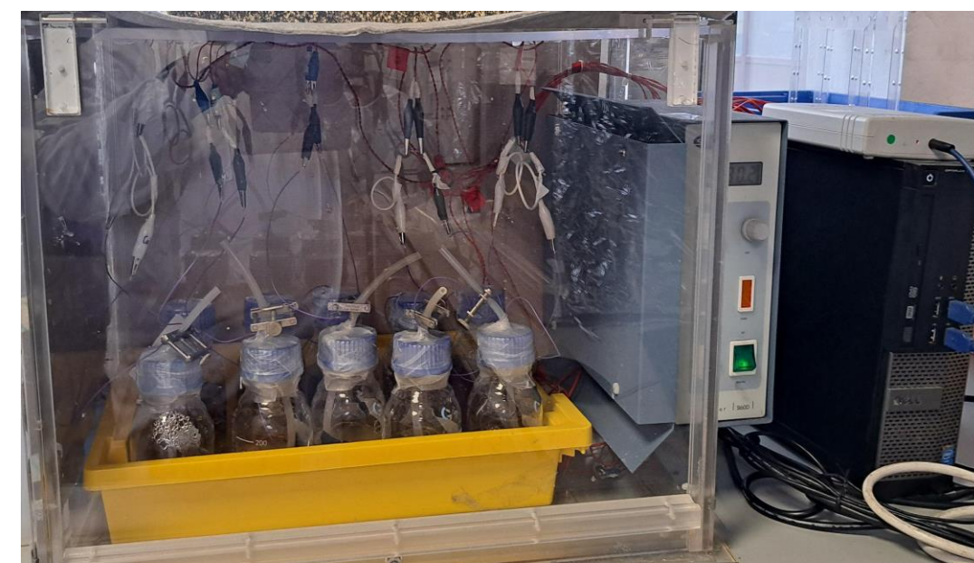
Figure 1d shows the laboratory setup of Microbial Fuel cells in an incubator.
